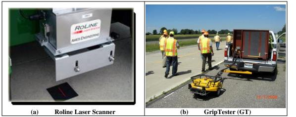
Figure 1. Devices for Collecting Texture and Friction Data: (a) Roline Laser Scanner for measuring profile and texture; (b) GripTester for measuring continuous friction.
