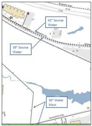
NNNW existing waterlines will be relocated to accommodate new bridge foundations as well as avoid the railroad lines.
