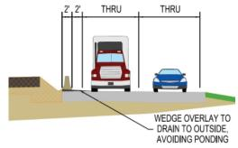
Figure 3.5.4 Example of Maintenance of Temporary Drainage
