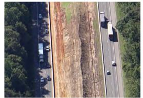
Figure 2 - Provided full shoulders during median widening on I-64 Capacity Improvements Segment III Project
