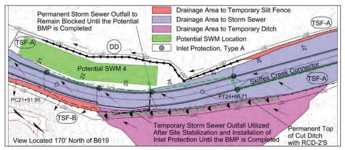
Figure 4.3.1.5 Erosion and Sediment Control Phase 3 to be Utilized while Constructing Potential SWM
