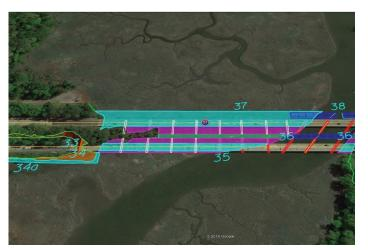
Figure 4.4.1.3 – Example of I-64 Segment III Capacity Improvements KMZ detailing impact areas over Queen's Creek. Impact number labels are utilized during VWP Permit Construction Compliance Inspections.
