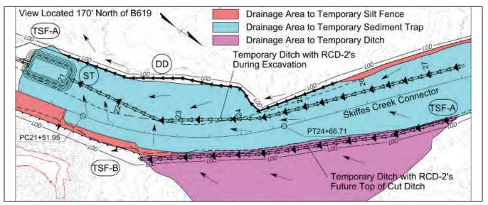
Figure 4.3.1.4 Erosion and Sediment Control Phase 2 to be Utilized During Major Grading
