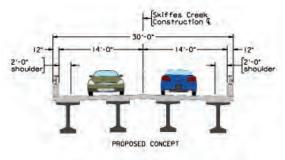
Figure 4.3.2.1 Transverse Section (B619)/B620
