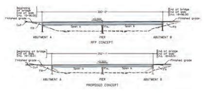
Figure 4.3.2.2 Bridge Span Comparison
