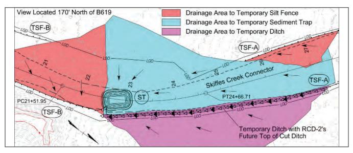
Figure 4.3.1.3 - Erosion and Sediment Control Phase 1 to be Utilized while Clearing and Initial Grading
