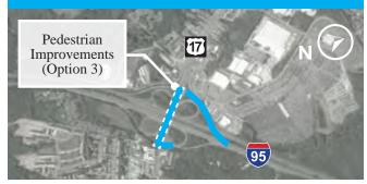
NB Route 17 will require a minor shift to the inside to allow for the widening and tie in to occur. In this phase, work can also begin along Route 17 Ramp B. Lanes here be will required to be reduced to 14' to allow for the proposed construction to occur.
