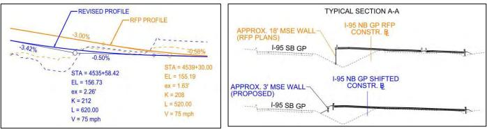
Figure 4.3.1.3: Proposed improved vertical profile of I-95 NB GP Lanes south of the Rappahannock River allowing for reduced retaining wall height and length.
