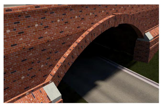
Figure 4.3.8: Colonial Parkway Aesthetics. Our design uses solid brick to blend the new portions of the widened arches with the existing arches.
