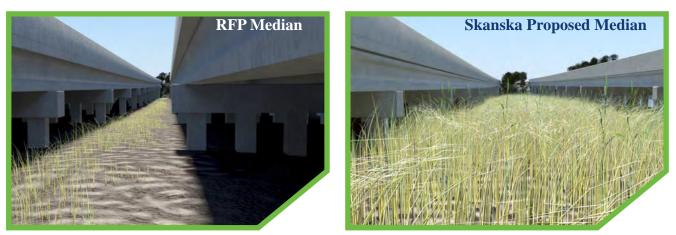
**Figure 4.4.: Queens Creek Median Alignment Shift (RFP vs Alignment Shift):** An upland area (8,400 square feet) between the shifted bridges can be regraded to the appropriate marsh elevation following completion of bridge construction, resulting in 30 percent less wetland footprint for the crossing.
