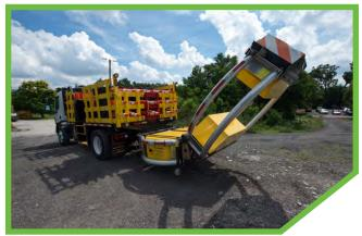
**Figure 4.5.21: Custom Designed MOT Trucks:** Skanska's specifically designed MOT trucks feature a basket that hydraulically adjusts up and down to make retrieving and laying cones safer and easier. The trucks are equipped with a custom interior video and intercom system to allow the driver to communicate and monitor the crew around the truck from the cab without turning around.
