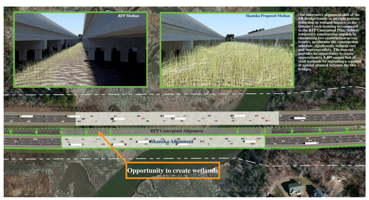
Figure 4.3.6: Bridge Replacement at I-64 over Queens Creek. Our proposed I-64 alignment is shifted 25 feet at Queens Creek and allows for more sunlight to the wetlands through a wider median. Virginia Department of Transportation -I-64 Capacity Improvements, Segment III – 4.3. Design Concept
