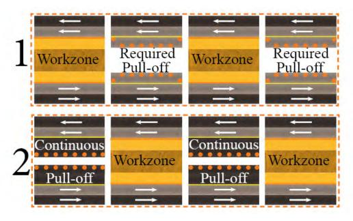
**Figure 4.5.9: Work zones and Pull-Off Cells.** Our SOC uses alternating mile-long work cells to advance construction, optimizing efficiency, working conditions, opportunities for recycling pavement materials, quality control, erosion control, and public safety.
