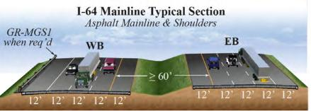
**Figure 4.3.1: Asphalt Mainline and Shoulders.** This typical section offers an environmentally conscious and economical solution.
