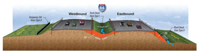
Figure 4.4.8: Reconstructing of Slope. The Skanska Team will use slope stability checks to ensure that the roadway, work zone, and utilities are safe and secured.
