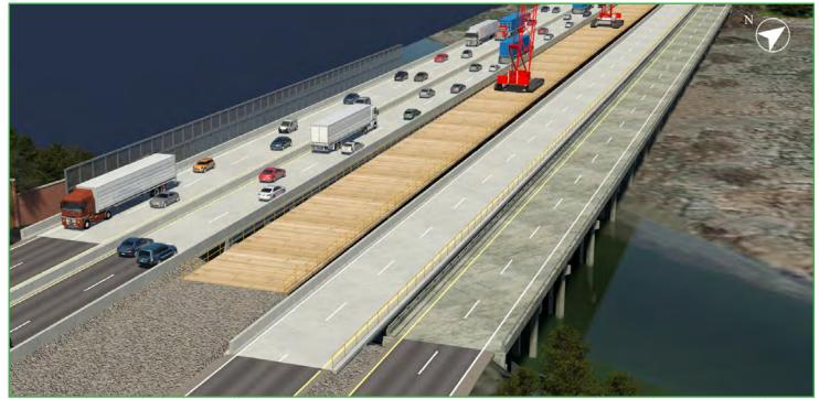
Figure 4.7.13: Phase 3 - Shift all traffic from WB bridges onto new EB bridge using temp median. Barrier wall and modified median crossovers. Enter Phase 3.
