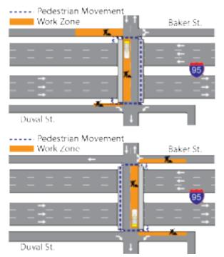
Figure 4.5.2-5 Proposed 1st St. Vehicle and Pedestrian Movements
