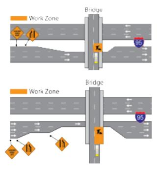
Figure 4.5.2-1 Typical lane closures for deck and beam removal over one direction of I-95
