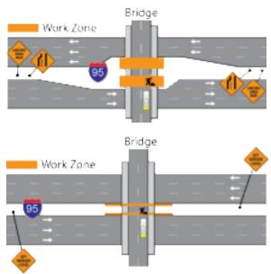
Figure 4.5.2-2 Typical phasing for pier repairs along I-95
