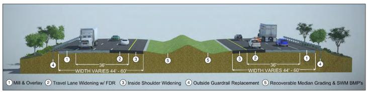
Figure 4.3.1-3: I-81 Typical Section
