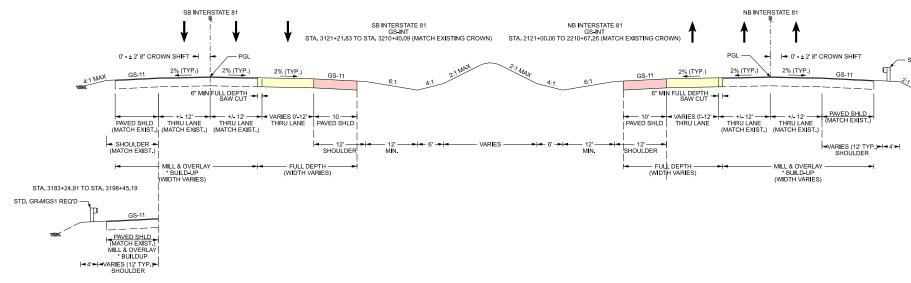
NOTES: 1. PROPOSED MINIMUM PAVEMENT SECTION IS TO BE IN ACCORDANCE WITH THE RFP SECTION 2.6.1.1 NEW PAVEMENT AND PAVEMENT WIDENING. 2. REHABILITATION OF EXISTING 1541 TRAVEL LANES IS TO BE IN ACCORDANCE WITH THE RFP SECTION 2.2 AND ATTACHMENT 2.6.1.2 3. ALL CURVES TO BE SUPERELEVATED IN ACCORDANCE WITH TC-5.11R UNLESS OTHERWISE NOTED AND ALLOWED BY THE RFP.
