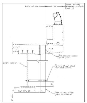
Figure 4.3.2-2: Example Temporary Scupper Detail
