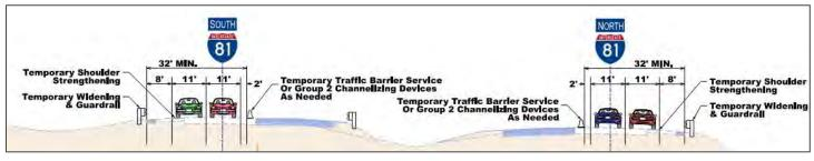
Figure 4.5.1-3: Phase 1 Typical Section
