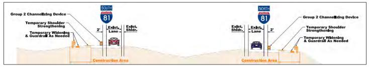
Figure 4.5.1-2: Advanced Work Package/Pre-Phase Typical Section
