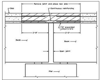
Figure 4.3.2-3: VDOT Flexible Link Slab
