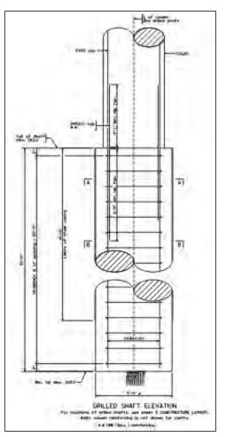
Figure 4.3.2-1: Example Drilled Shaft
