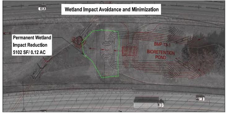
Figure 4.4.1-1: Wetland Impact Avoidance and Minimization
