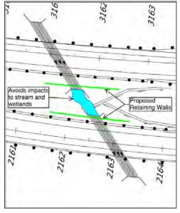
Figure 4.3.1-4: Box Culvert Extension Elimination
