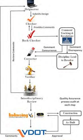
Figure 4.4.4-1: Design QA/QC Workflow Diagram
