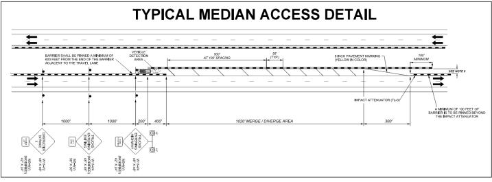
Figure 4.5.2-2: Typical Construction Ingress/Egress
