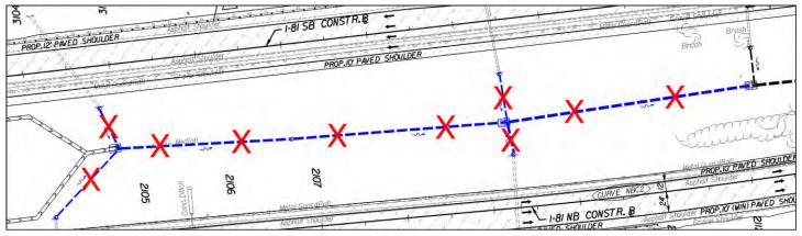
*Figure 4.3.1-6: Proposed Storm Sewer Elimination*
