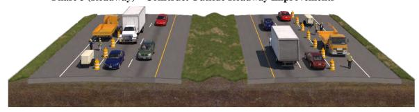
Phase 4 (Roadway) – Perform Mill and Overlay and Final Signing and Striping
