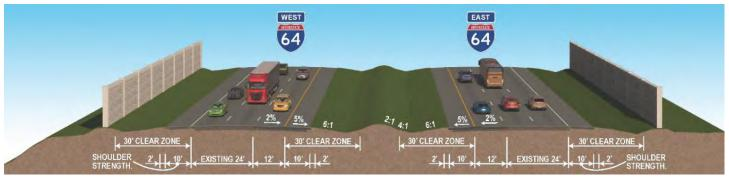
Figure 4.3.1-3: Proposed Roadway Typical Section
