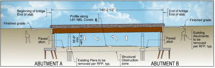
Figure 3 – Bridge Developed Section
