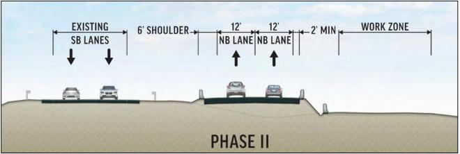
Figure 9 – Phase II Section AA Work Zone
