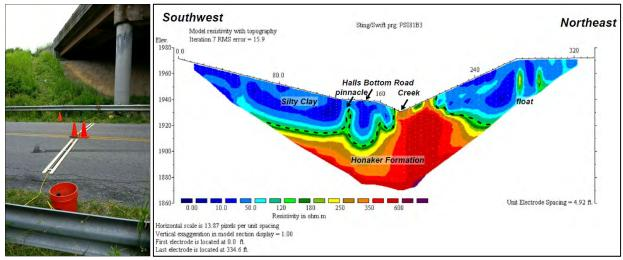
Figure 4 - Electric Resistivity Plot for I-81 Over Sinking Creek and Halls Bottom Road
