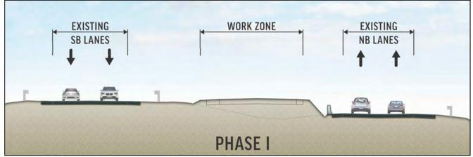
Figure 7 – Phase I Section AA Work Zone
