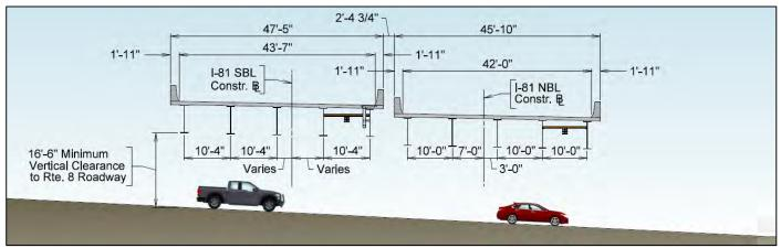
Figure 2 – Bridge Transverse Section
