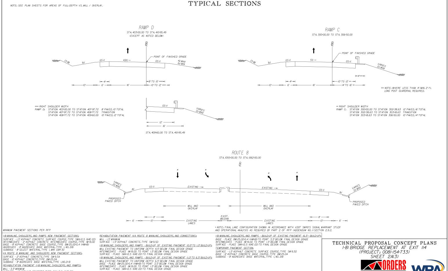
MILL - 3.5 MINIMUM SURFACE - 1.5" ASPHALT CONCRETE, TYPE SMA-12.5 (64E-22) INTERMEDIATE - 2" ASPHALT CONCRETE, TYPE IM-19.0D
