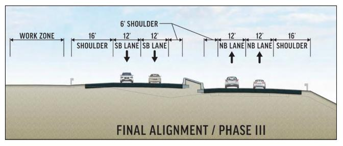
Figure 11 – Phase III Section AA Work Zone
