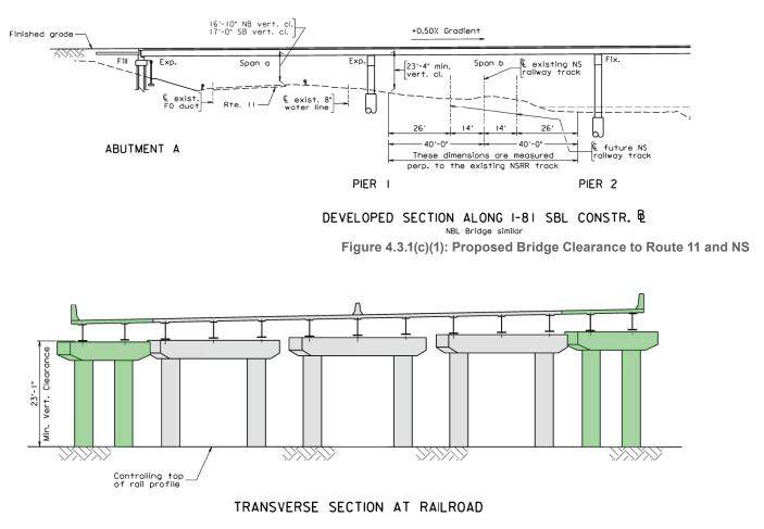
Figure 4.3.1(c)(2): Future Widened Bridge (Green) Clearance to NS Top of Rail
