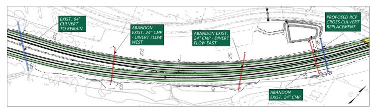
Figure 4.3.1(e)(1): Concept to Abandon Two of the Three Existing Major Cross-Culverts
