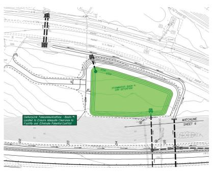
Figure 4.3.1(e)(2): Proposed Stormwater Facility
