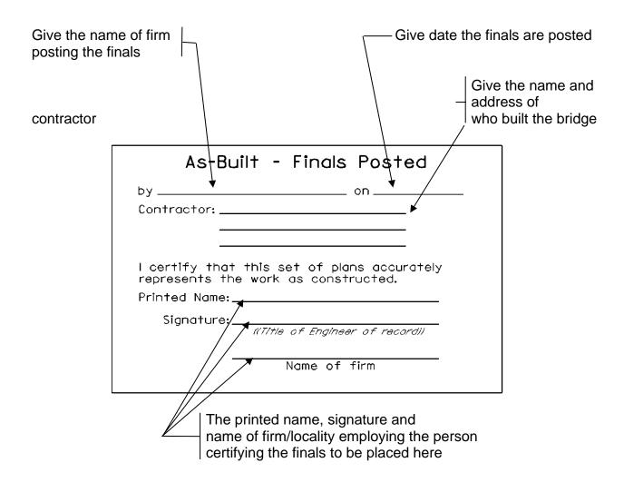
This block and information shown shall be located on the title sheet of each set of bridge plans certifying that the as-built plans accurately reflect the final product.
