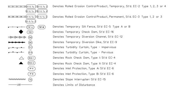
The ESC symbols are to be used to denote proposed erosion and sediment control items on the plans and are available in the CADD Cell and Custom Line Style Libraries and the GEOPAK Road Plan View Labels.
