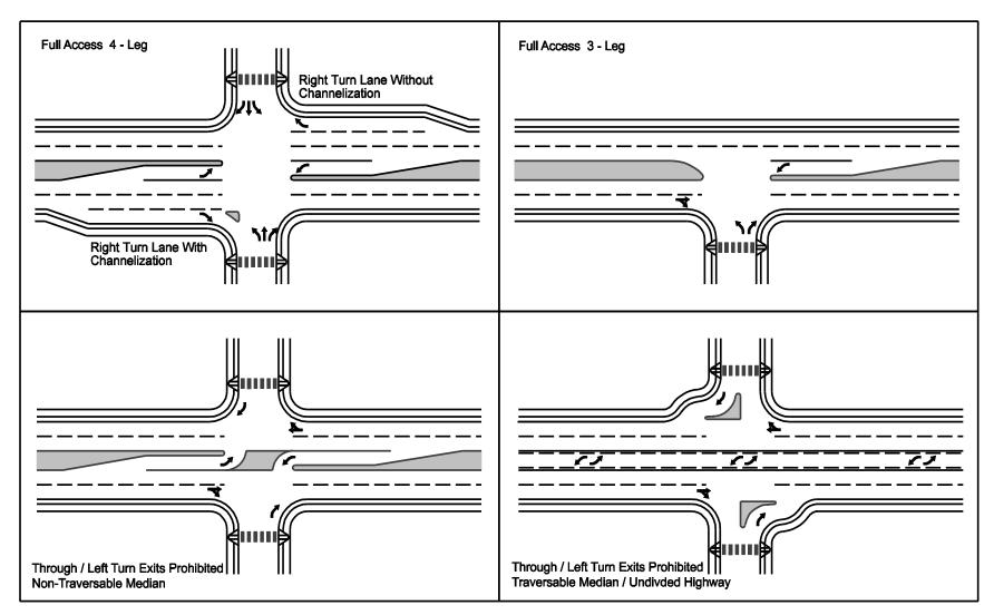
FIGURE 2-3 TYPES OF ACCESS CHANNELIZATION
