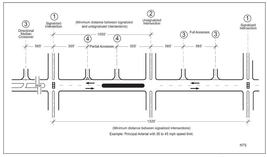
FIGURE 2-8.1 ILLUSTRATION OF THE RELATIONSHIP BETWEEN SPACING STANDARDS
