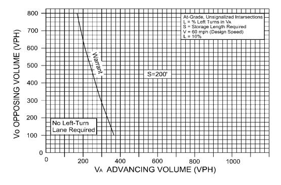
FIGURE 3-17 WARRANT FOR LEFT TURN STORAGE LANES ON TWO LANE HIGHWAY
