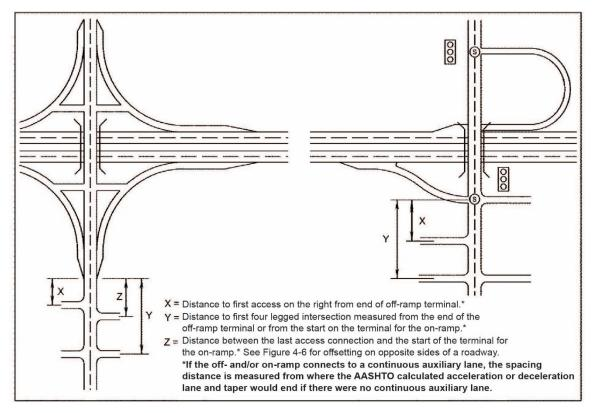
FIGURE 2-10 ACCESS CONTROL ON TWO-LANE CROSSROADS AT INTERCHANGES
