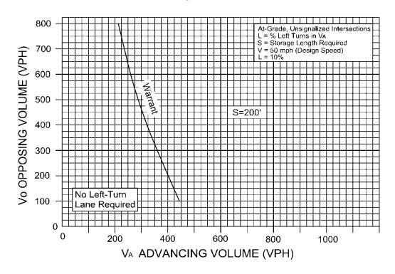
FIGURE 3-11 WARRANT FOR LEFT TURN STORAGE LANES ON TWO LANE HIGHWAY
