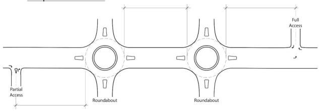
When determining the distance between a roundabout and another access, the measurement is not taken from the centerline. Instead, the point of reference is the outer edge of the inscribed circle diameter (Yield Line) on the nearest approach.
