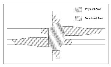
FIGURE 4-2A PHYSICAL AND FUNCTIONAL AREAS OF INTERSECTION
