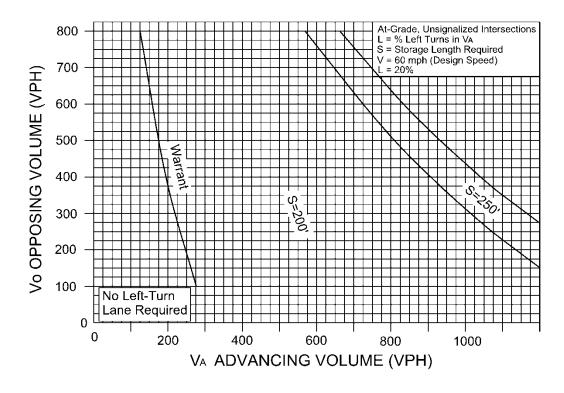
FIGURE 3-19 WARRANT FOR LEFT TURN STORAGE LANES ON TWO LANE HIGHWAY
