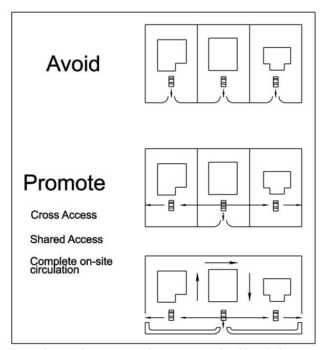
FIGURE 4-7 SHARED ENTRANCE AND INTERNAL SITE CONNECTION
