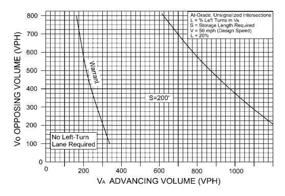
FIGURE 3-13 WARRANT FOR LEFT TURN STORAGE LANES ON TWO LANE HIGHWAY
