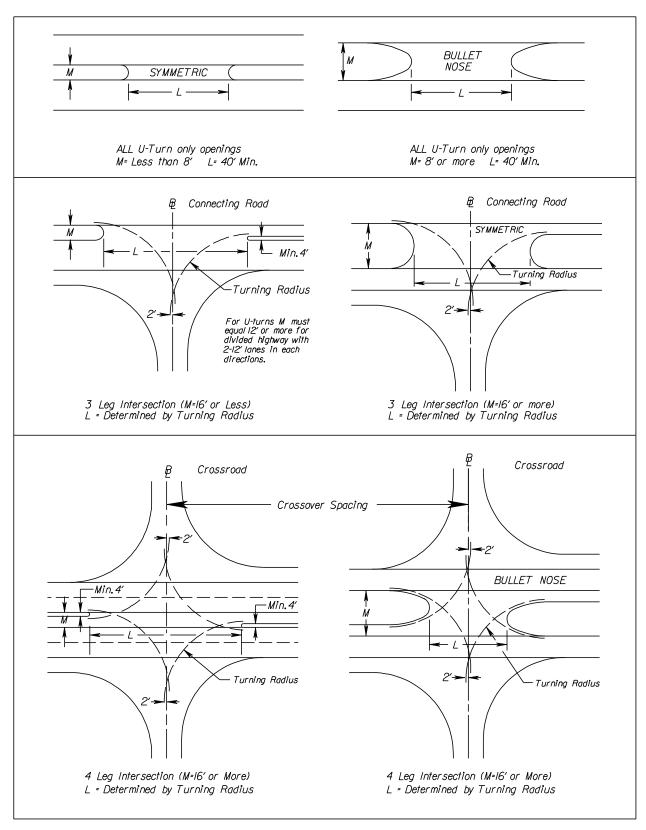
FIGURE 2-13 MEDIAN CROSSOVERS WITH AND WITHOUT CONNECTIONS\*
