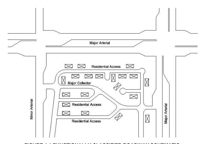
FIGURE 1-1 FUNCTIONALLY CLASSIFIED ROADWAY SCHEMATIC
