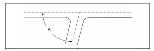
FIGURE 2-6 MINIMUM ANGLE OF INTERSECTIONS
