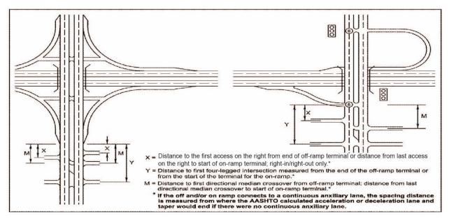
FIGURE 2-9 ACCESS CONTROL ON MULTILANE CROSSROADS AT INTERCHANGES
