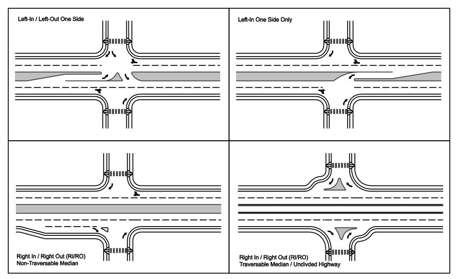
FIGURE 2-4 TYPES OF ACCESS CHANNELIZATION
