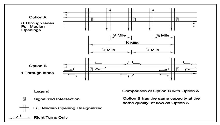
FIGURE 2-8 ILLUSTRATION OF ENTRANCE AND INTERSECTION SPACING
