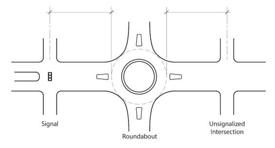
Type 4 Spacing – Spacing from roundabouts to other roundabouts, full accesses, and partial accesses.\*
