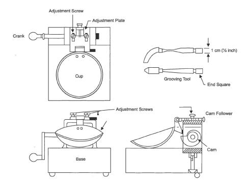
4. <u>Obtain a sample weighing approximately 50 grams</u> from the thoroughly mixed portion of the material passing the No. 40 (425 μm) sieve. Place this material in a mixing dish and mix with 8-10 ml of distilled or demineralized water. The material is mixed by alternately and repeatedly stirring, kneading, and chopping with a spatula. If additional water is needed in the mixture, it shall be added increments of 1-3 ml. It shall then be thoroughly mixed in stiff consistency.
