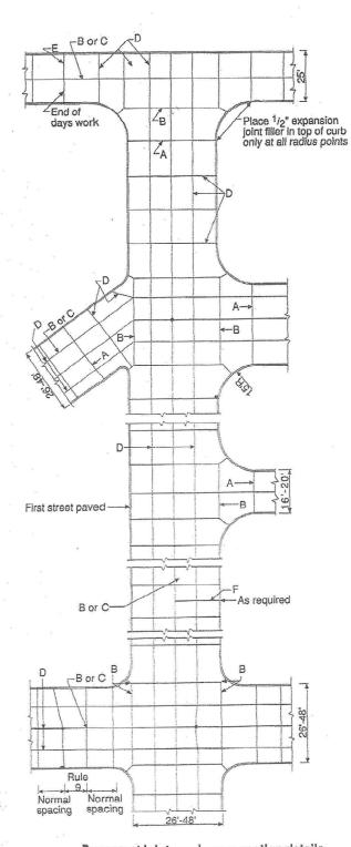
Pavement joints and cross section details
