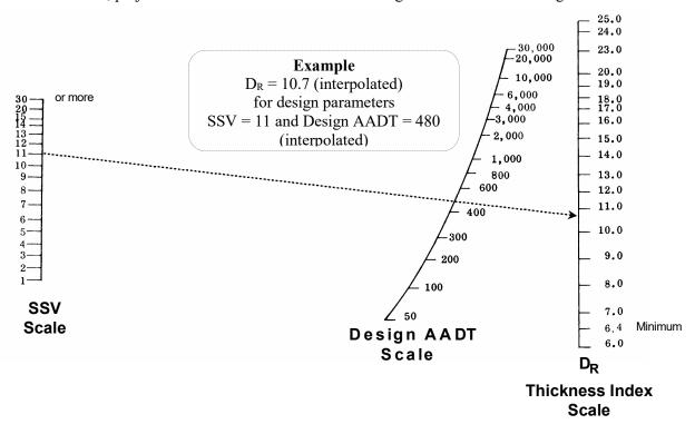
The nomograph depicted correlates the soil support value of the subgrade (SSV = Design CBR x RF), the traffic volume (Design AADT), and the minimum required pavement design thickness index ( $D_R$ ) for subdivision streets and secondary road pavement, based on AASHO design equations. The equation on which the nomograph is based is:  $D_R = 3.48$ Ln (AADT) – 1.48Ln (SSV) - 7.23, where Ln is the natural logarithm. This nomograph assumes the following:
