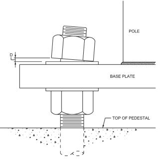
Figure 6.3 Measurement Methodology for Improperly Seated Nuts
