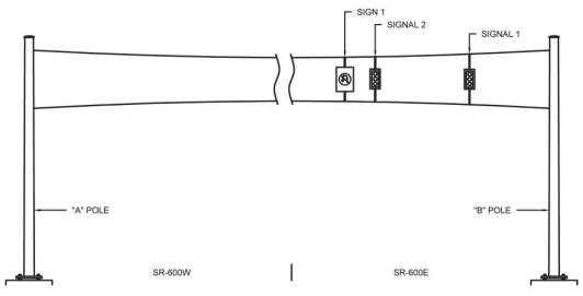
Figure 5.24 Methodology for Four Pole Span Wire, Span Wire Distribution Elevation
