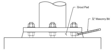
Figure 6.4 Method for Drilling Grout Pad to Determine Existence of Leveling Nuts
