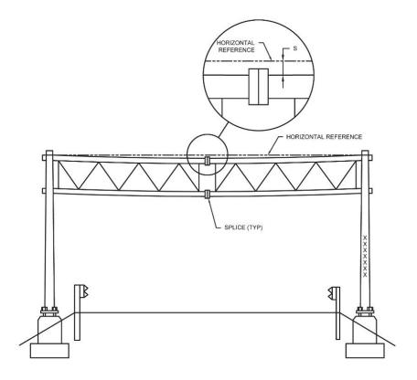
Figure 4.12 Measurement Methodology for Chord Sag
