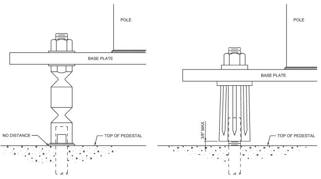
Figure 6.10 Distance between Top of Pedestal and Bottom of Coupler
