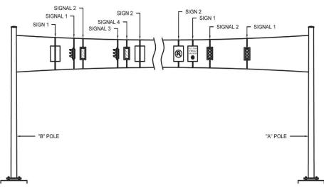
Figure 5.21 Methodology for Two Pole Span Wire, Span Wire Distribution Elevation
