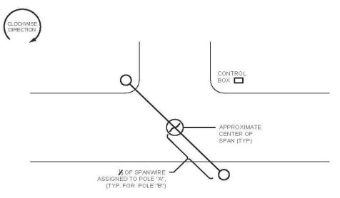
Figure 5.20 Methodology for Two Pole Span Wire, Span Wire Distribution Plan
