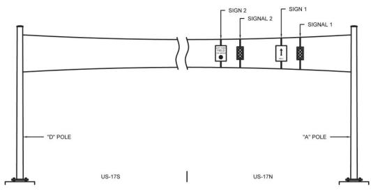
Figure 5.23 Methodology for Four Pole Span Wire, Span Wire Distribution Elevation
