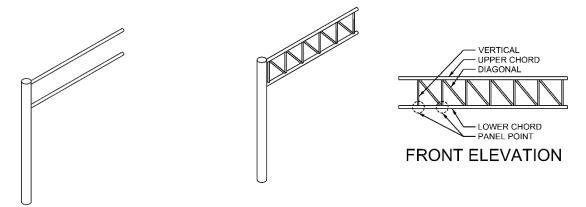
Figure 1.22 Cantilever, Two Chord, Untrussed
