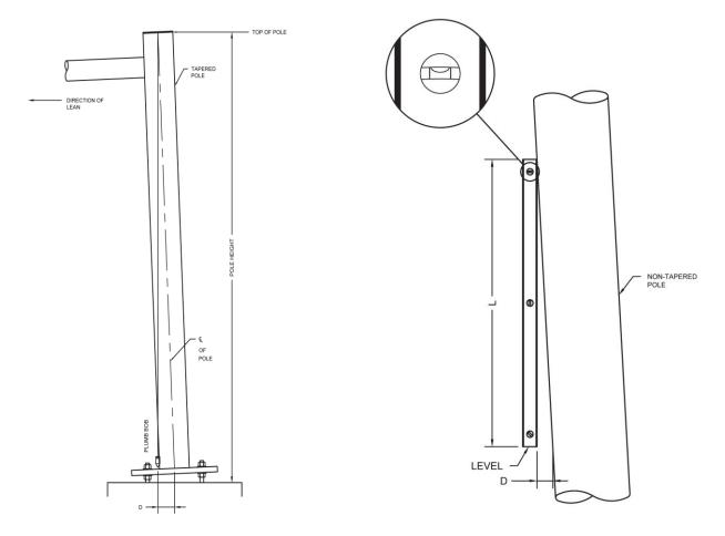
Figure 6.15 Measurement Methodology for Leaning or Out of Plumb Tapered Poles
