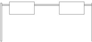
Figure 1.5 Overhead Span, Single Chord and Pole Structure
