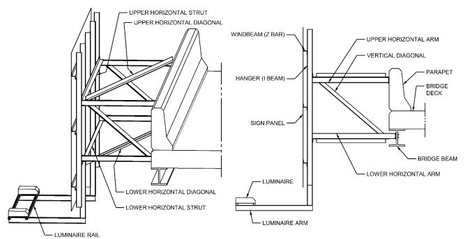
Figure 1.34 Bridge Parapet Mount Signs
