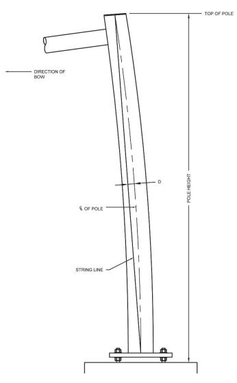
Figure 5.10 Measurement Methodology for Bowed Poles
