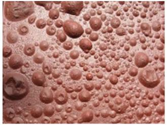
Photo 3.22 Coating failure with blistering paint
