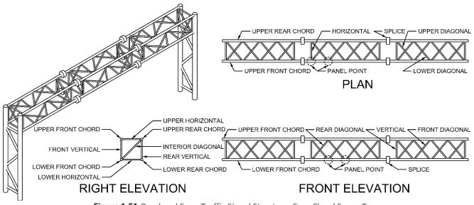
Figure 1.51 Overhead Span Traffic Signal Structure, Four Chord Space Truss
