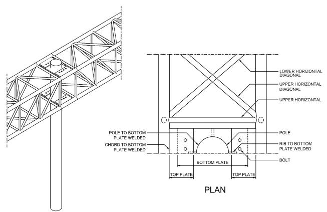
Figure 1.33 Butterfly Chord to Pole Connection, Collar Plate, Tubular
