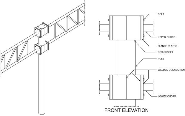
Figure 1.32 Butterfly Chord to Pole Connection, Gusseted Box Flange Plates
