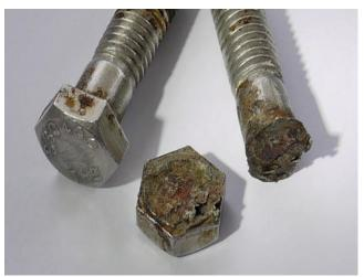
Photo 3.27 Broken stainless steel bolt
