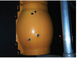
Photo 5.100 Bullet holes in backside of signal head
