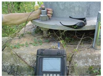
Photo 2.1 Ultrasonic testing of an anchor bolt
