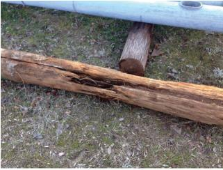
Photo 6.54 Decay below grade, shown after pole removal
