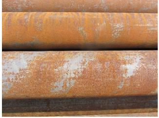
Photo 3.16 Corrosion with no section loss
