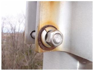
**Photo 3.39** Galvanic corrosion of galvanized washer due to stainless steel bolt assembly
