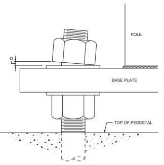
Figure 4.3 Measurement Methodology for Improperly Seated Nuts
