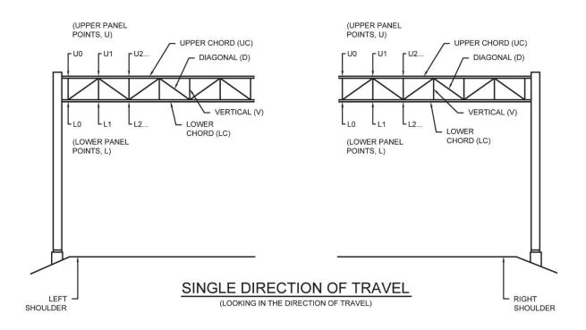
**Figure 4.35** Methodology for Panel Point Numbering and Component Labeling of Cantilever (Two Chord and Four Chord Truss) Sign Structures
