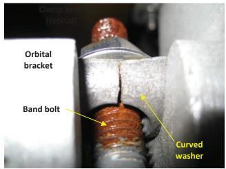
**Photo 5.80** Broken curved washer at band bolt to orbital bracket connection
