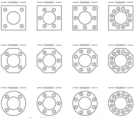
Figure 6.24 Anchor Bolt Numbering Methodology
