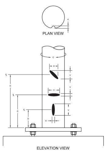
Figure 5.11 Measurement Methodology for Dents and Ruptures in Round or Faceted Poles
