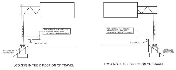
Figure 4.15 Cantilever Sign Structures, Number and GPS Locations, At Structure (Looking in Direction of Travel)
