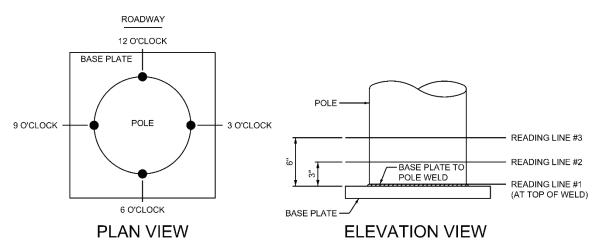
Figure 6.13 Measurement Methodology for Pole Corrosion Thickness Gage Readings, Plan and Elevation
