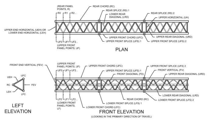
Figure 4.31 Methodology for Panel Point Numbering and Component Labeling of Tri-Chord Truss Sign Structures with Splices
