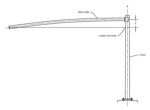
*Figure 5.12 Measurement Methodology for Mast Arm Sag*
