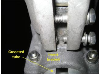
Photo 5.82 1 of 2 clamp bolts broken at orbital bracket
