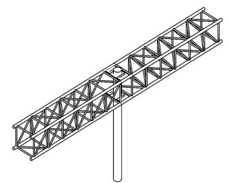
Figure 1.28 Butterfly, four chord box truss
