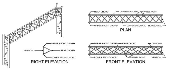
Figure 1.8 Overhead Span, Tri-Chord Space Truss
