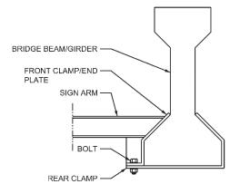
Figure 1.39 Attachment to Bridge Beam, Saddle Clamp
