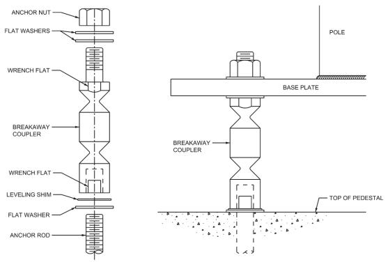
Figure 6.6 Typical Steel Double Neck Coupler Assembly
