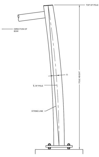
Figure 4.10 Measurement Methodology for Bowed Poles
