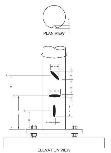
Figure 4.11 Measurement Methodology for Dents and Ruptures in Round or Faceted Poles
