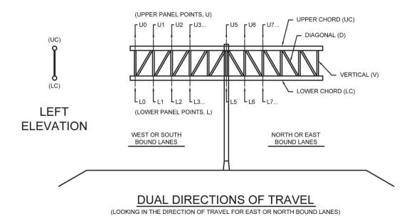
**Figure 4.34** Methodology for Panel Point Numbering and Component Labeling of Butterfly (Two Chord Truss) Sign Structures
