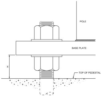
Figure 5.5 Measurement Methodology for Base Plate Distance Above Pedestal
