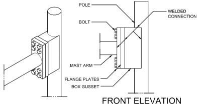
Figure 1.44 Mast arm to pole connection
