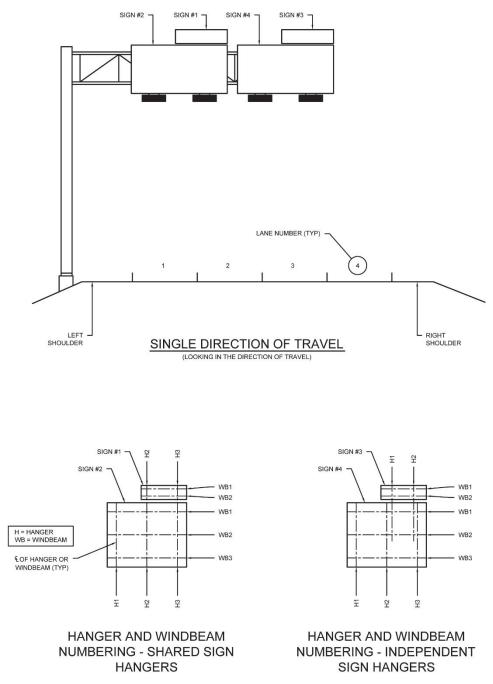
**Figure 4.24** Methodology for Sign Panel and Component (Windbeam/Hanger) Numbering of Left Side Cantilever Sign Structures without a Median or Barrier
