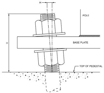
Figure 5.2 Measurement Methodology for Out of Plumb Anchor Bolts
