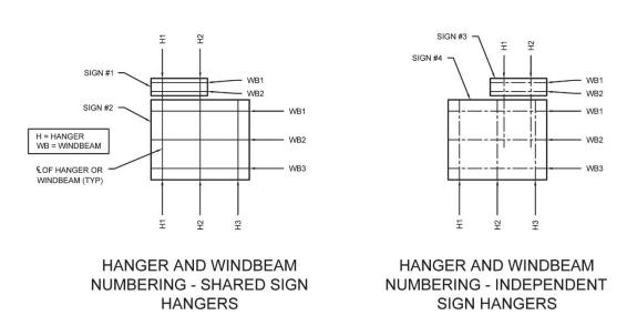
**Figure 4.25** Methodology for Sign Panel and Component (Windbeam/Hanger) Numbering of Butterfly Sign Structures without a Median or Barrier
