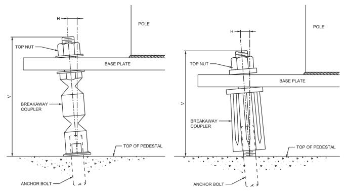
Figure 6.8 Measurement Methodology for Out of Plumb Coupler Assembly
