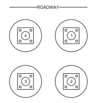
Figure 6.23 Methodology for Cell Tower Base Numbering and Pole Labeling
