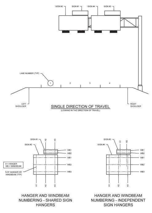
**Figure 4.23** Methodology for Sign Panel and Component (Windbeam/Hanger) Numbering of Right Side Cantilever Sign Structures without a Median or Barrier
