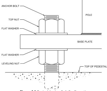
Figure 4.1 Typical Anchor Bolt Configuration
