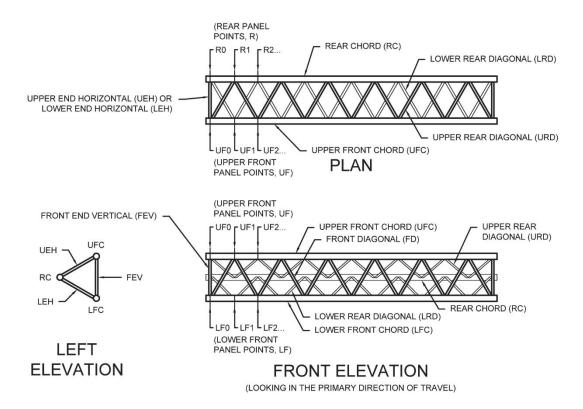
*Figure 4.30* Methodology for Panel Point Numbering and Component Labeling of Tri-Chord Truss Sign Structures without Splices
