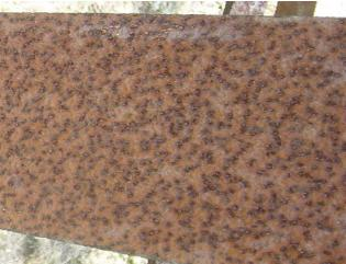
Photo 3.17 Corrosion with pitting
