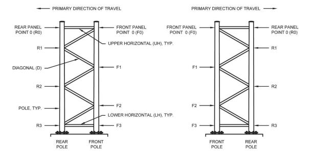
*Figure 4.36 Methodology for Panel Point Numbering of Trussed Vertical Supports (End Frames)*
