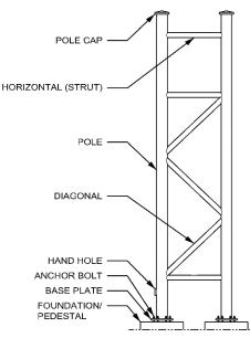
Figure 1.14 Two Pole Truss (End Frame), Elevation
