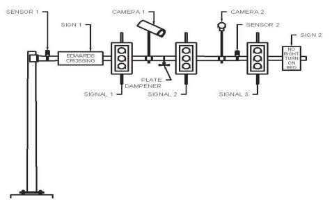
*Figure 5.19* Methodology for Signal Head and Attachment Labeling/Numbering with Pole on Left Side of Roadway
