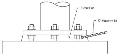
*Figure 4.4* Method for Drilling Grout Pad to Determine Existence of Leveling Nuts
