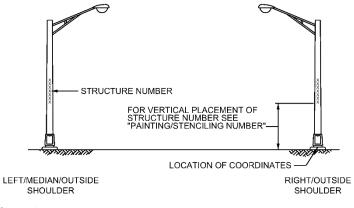
**Figure 6.20** Pole Structures, Number and GPS Locations, At Structure (Looking in Direction of Traffic)
