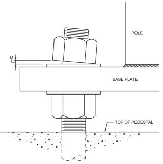
Figure 5.3 Measurement Methodology for Improperly Seated Nuts
