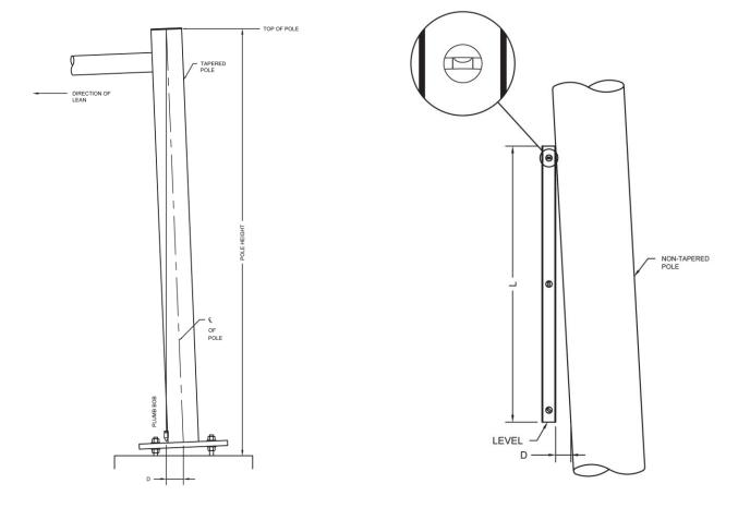
Figure 5.8 Measurement Methodology for Leaning or Out of Plumb Tapered Poles
