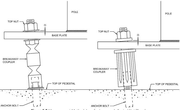
Figure 6.9 Measurement Methodology for Improperly Seated Nut/Coupler
