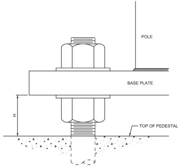
Figure 4.5 Measurement Methodology for Base Plate Distance Above Pedestal
