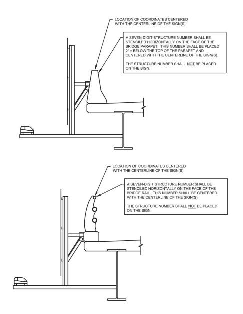
Figure 4.17 Bridge Parapet Mount Sign Structure, Number and GPS Locations
