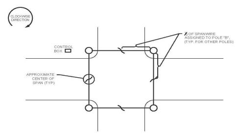
Figure 5.22 Methodology for Four Pole Span Wire, Span Wire Distribution Plan
