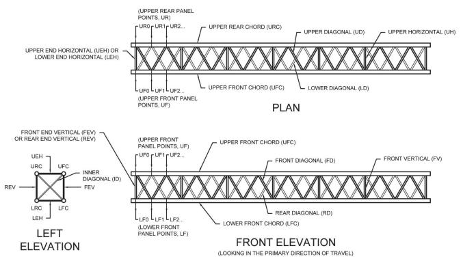
**Figure 4.32** Methodology for Panel Point Numbering and Component Labeling of Four Chord Truss Overhead Span and Cantilever Sign Structures without Splices
