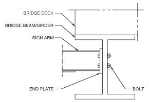
Figure 1.38 Attachment to Bridge Beam, Through Bolt
