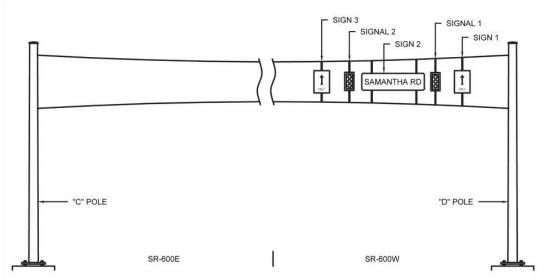
Figure 5.26 Methodology for Four Pole Span Wire, Span Wire Distribution Elevation
