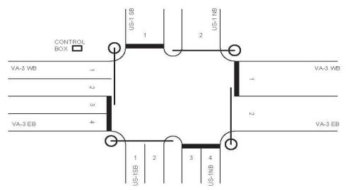
Figure 5.14 Methodology for Lane Numbering with US-1 as the Primary Route and VA-3 as the Secondary Route
