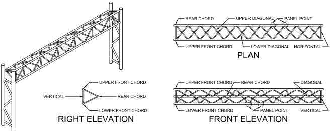
Figure 1.50 Overhead Span Traffic Signal Structure, Tri-Chord Space Truss
