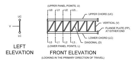
Figure 4.29 Methodology for Panel Point Numbering and Component Labeling of Two Chord Truss Sign Structures without Splices
