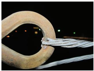
Photo 5.62 Broken strands on span wire at connection to pole
