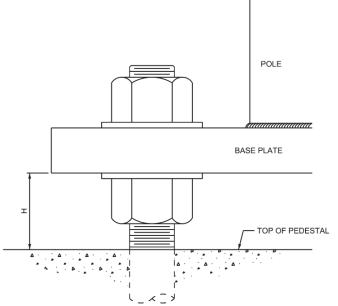
*Figure 6.5 Measurement Methodology for Base Plate Distance Above Pedestal*
