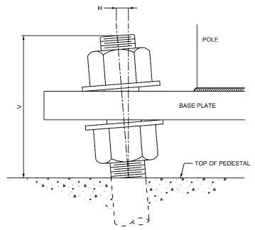
Figure 6.2 Measurement Methodology for Out of Plumb Anchor Bolts
