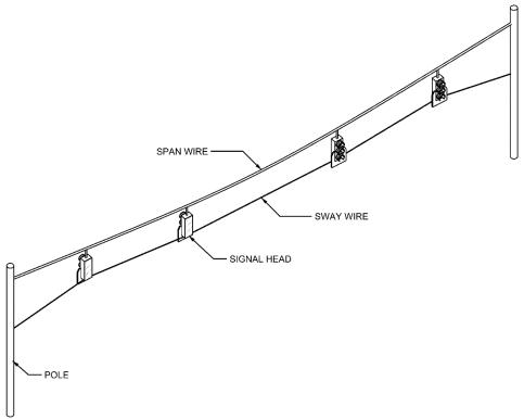
Figure 1.45 Span Wire Traffic Signal Structure
