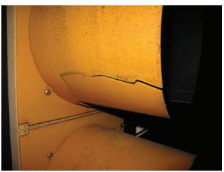
Photo 5.98 Broken visor on signal head
