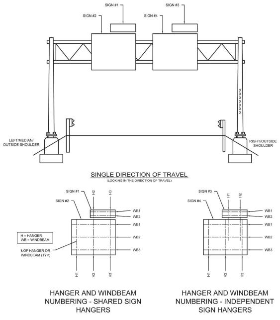
**Figure 4.21** Methodology for Sign Panel and Component (Windbeam/Hanger) Numbering of Overhead Sign Structures without a Median or Barrier
