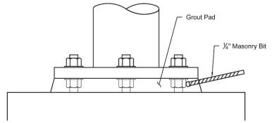
Figure 5.4 Method for Drilling Grout Pad to Determine Existence of Leveling Nuts
