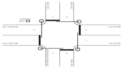
Figure 5.13 Methodology for Lane Numbering with US-1 as the Primary Route and US-17 Bus as the Secondary Route
