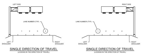
*Figure 4.19* Methodology for Lane Numbering of Cantilever Sign Structures
