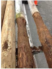
Photo 5.48 Decay below grade, shown after pole removal
