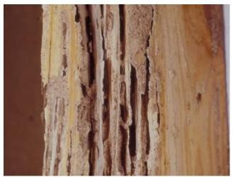
Photo 3.13 Insect damage (termite)
