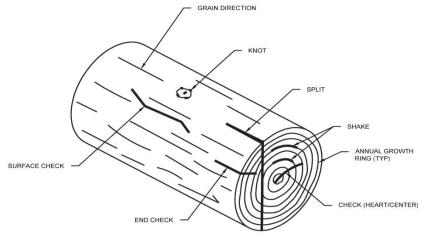
Figure 3.1 Typical Timber Defects
