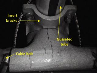
Photo 5.79 Crack in orbital bracket
