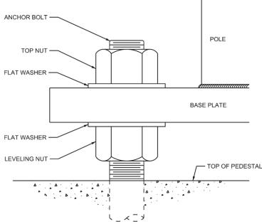
Figure 6.1 Typical Anchor Bolt Configuration
