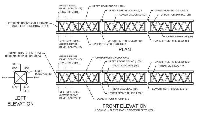
**Figure 4.33** Methodology for Panel Point Numbering and Component Labeling of Four Chord Truss Overhead and Cantilever Sign Structures with Splices
