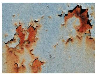
**Photo 3.23** Coating failure with peeling paint with underlying corrosion
