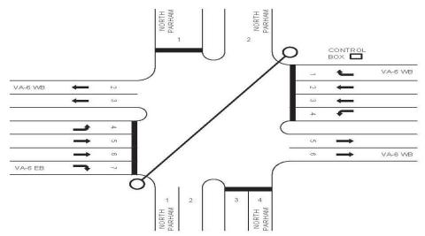
Figure 5.17 Methodology for Lane Numbering with US-1 as the Primary Route and US-17 as the Secondary Route
