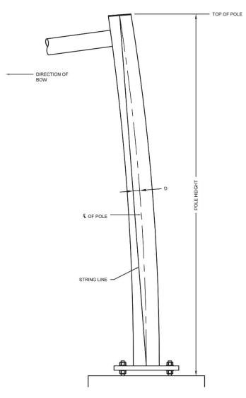
Figure 6.17 Measurement Methodology for Bowed Poles
