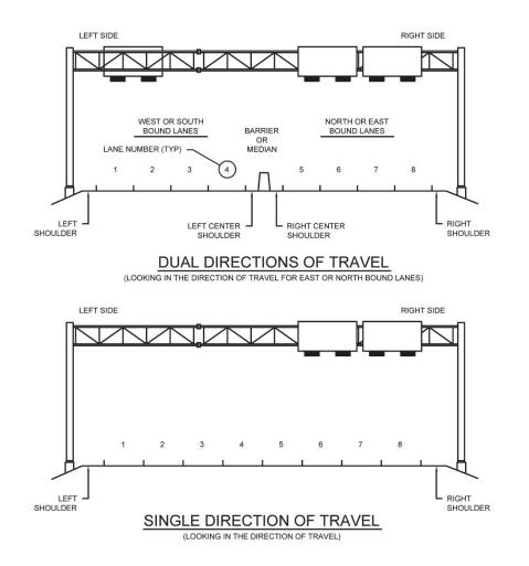
Figure 4.18 Methodology for Lane Numbering of Overhead Span Sign Structures
