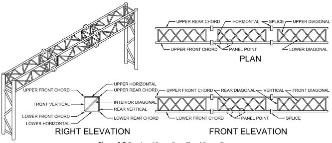
Figure 1.9 Overhead Span, Four Chord Space Truss
