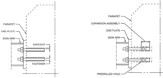
Figure 1.35 Adhesive Anchorage
