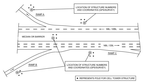
**Figure 6.19** Cell Tower Structures (Multi-Pole Shown), Number and GPS Locations (Single Direction of Traffic and Double Direction of Traffic)
