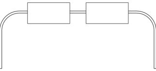
Figure 1.6 Overhead Span, Monotube Structure
