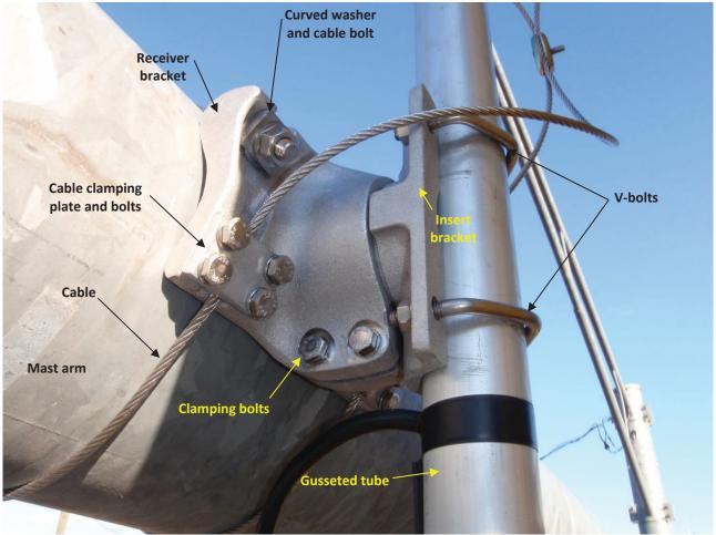
Photo 1.46 Typical orbital bracket
