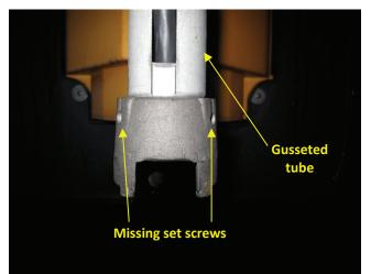
Photo 5.89 Missing set screws at lower gusseted tube connection
