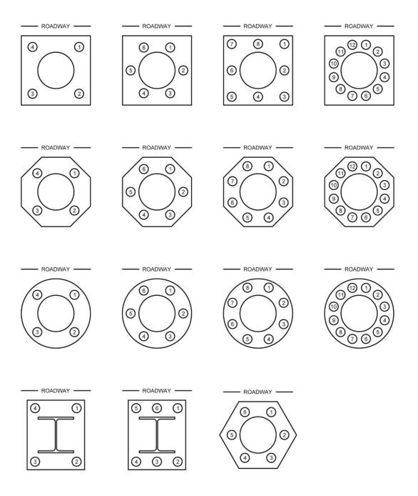
Figure 4.37 Anchor Bolt Numbering Methodology
