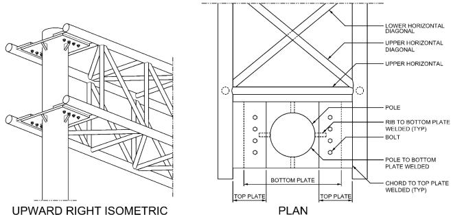
Figure 1.26 Cantilever Chord to Pole Connection, Collar Plate, Tubular Chords
