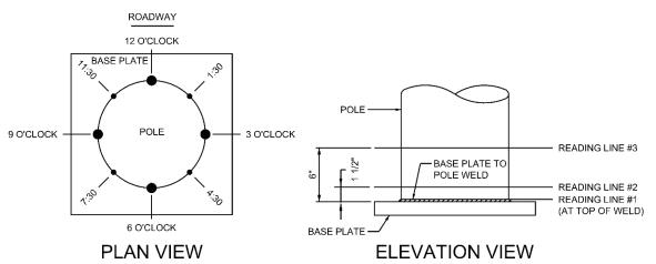
Figure 6.12 Measurement Methodology for High Mast Light Corrosion Thickness Gage Readings, Plan and Elevation
