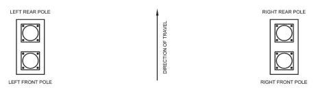
Figure 4.26 Methodology for Pole Labeling of Overhead Span Sign Structures without a Median Barrier
