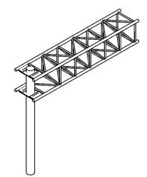
Figure 1.20 Cantilever, Four Chord Space Truss
