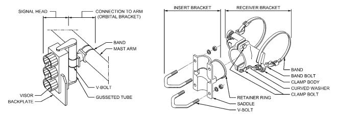
Figure 1.42 Traffic Signal Head
