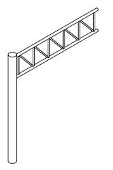
Figure 1.19 Cantilever, Two Chord Plane Truss
