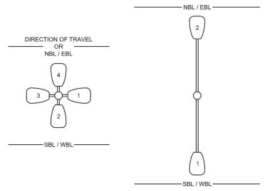
Figure 6.22 Methodology for Luminaire Head Numbering
