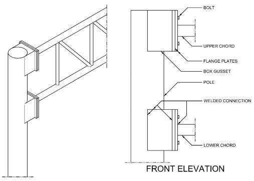
Figure 1.11 Overhead Span Chord to Pole Connection, Gusseted Box Flange Plates
