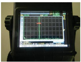
**Photo 2.2** Ultrasonic testing of an anchor bolt with an indication at 3.9" below top of the bolt
