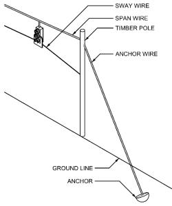
Figure 1.46 Timber Pole Anchorage
