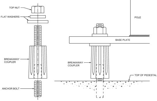
Figure 1.55 Typical Cast Aluminum Coupler Assembly
