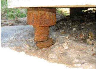
Photo 4.30 Corroded and broken anchor bolt
