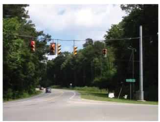
Photo 5.5 Front view of span wire governing two routes
