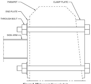
Figure 1.37 Parapet Through Bolt
