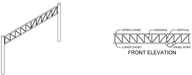
Figure 1.49 Overhead Span Traffic Signal Structure, Two Chord Plane Truss
