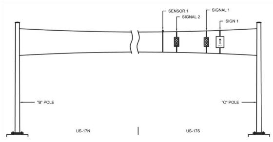
Figure 5.25 Methodology for Four Pole Span Wire, Span Wire Distribution Elevation
