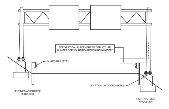
**Figure 4.13** Overhead Span Sign Structures, Number and GPS Locations, Overall (Single Direction of Traffic and Double Direction of Traffic)
