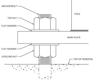
Figure 5.1 Typical Anchor Bolt Configuration
