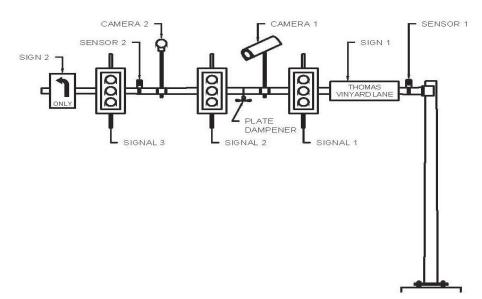
Figure 5.18 Methodology for Signal Head and Attachment Labeling/Numbering with Pole on Right Side of Roadway
