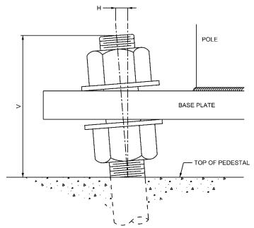
Figure 4.2 Measurement Methodology for Out of Plumb Anchor Bolts
