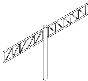
Figure 1.27 Butterfly, two chord planar truss
