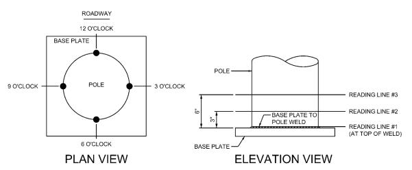
Figure 5.6 Measurement Methodology for Pole Corrosion Thickness Gage Readings, Plan and Elevation
