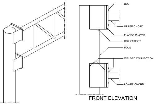
Figure 1.25 Cantilever Chord to Pole Connection, Gusseted Box Flange Plates
