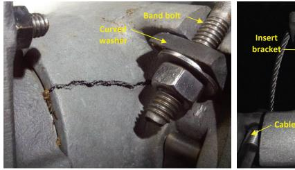
Photo 5.78 Crack in orbital bracket
