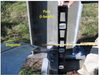
Photo 4.43 Measuring impact damage to pole diagonal
