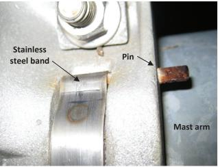
Photo 5.83 Zinc pin not fully seated at stainless steel band connection, note corrosion on pin
