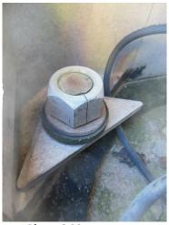
Photo 6.28 Cracked nut
