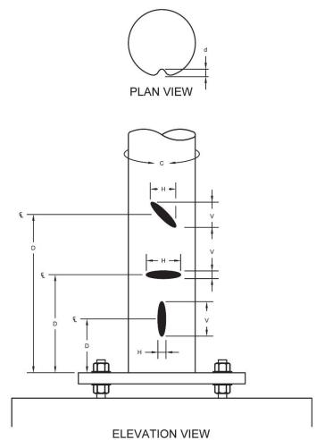
Figure 6.18 Measurement Methodology for Dents and Ruptures in Round or Faceted Poles
