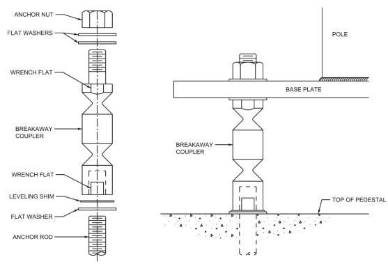
Figure 1.54 Typical Steel Double Neck Coupler Assembly
