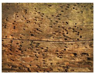
Photo 3.15 Insect damage (powder post beetles)
