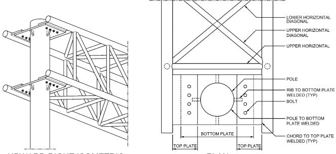
UPWARD RIGHT ISOMETRIC PLAN Figure 1.12 Overhead Span Chord to Pole Connection, Collar Plate, Tubular Chords
