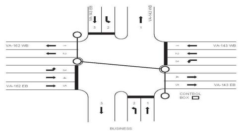
Figure 5.16 Methodology for Lane Numbering with VA-143 as the Primary Route and VA-162 as the Secondary Route
