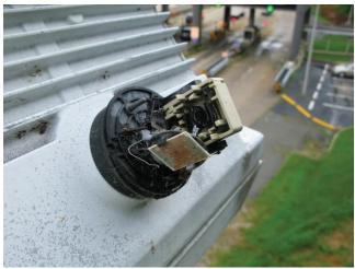
Photo 6.69 Photo sensor broken
