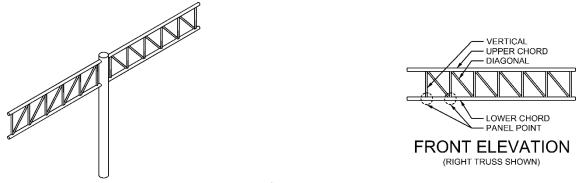
Figure 1.30 Butterfly, Two Chord Planar Truss
