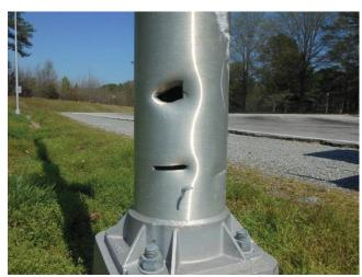
Photo 6.46 Impact damage to pole
