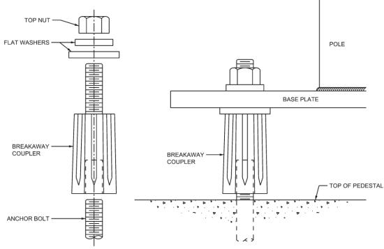
Figure 6.7 Typical Cast Aluminum Coupler Assembly
