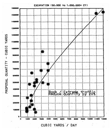
Figure 7: Maryland SHA Production Rate Curve for Excavation greater than 90k cy
