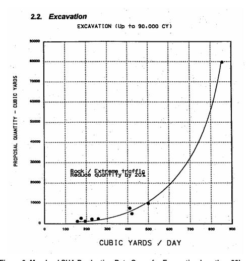
Figure 6: Maryland SHA Production Rate Curve for Excavation less than 90k cy
