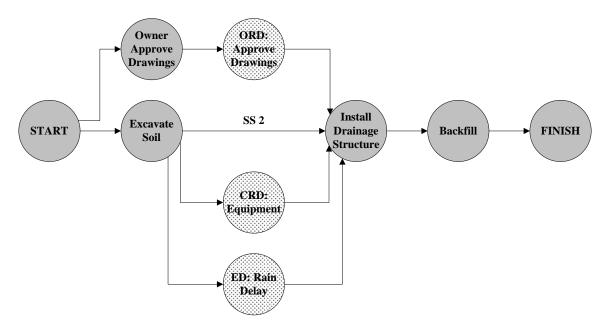
Figure 6: As-Built CPM Network for Drainage Structure Example
