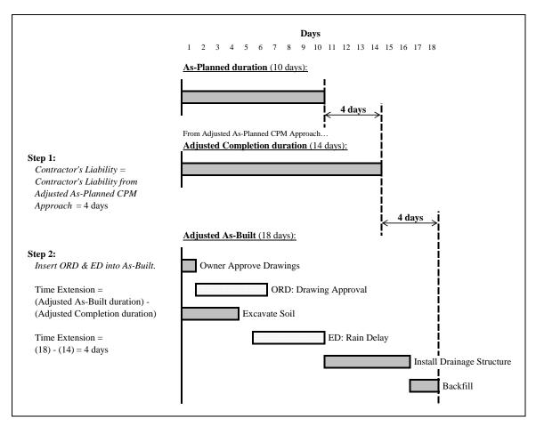
Figure 17: Adjusted As-Built CPM Approach
