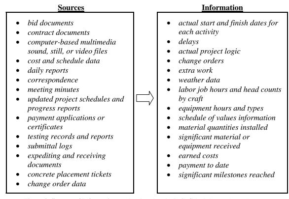
Figure 3: Sources of Information used to Develop As-Built Schedule [Knoke et al. 1996]
