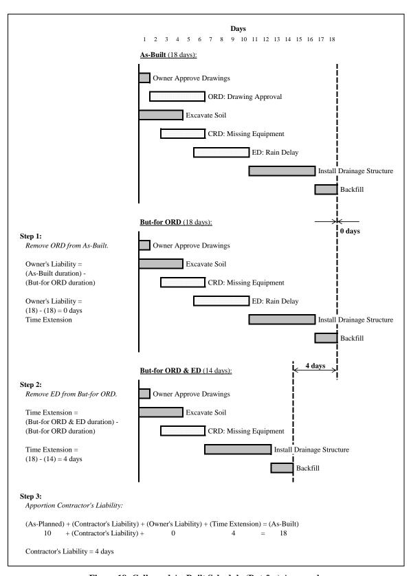
Figure 18: Collapsed As-Built Schedule (But-for) Approach
