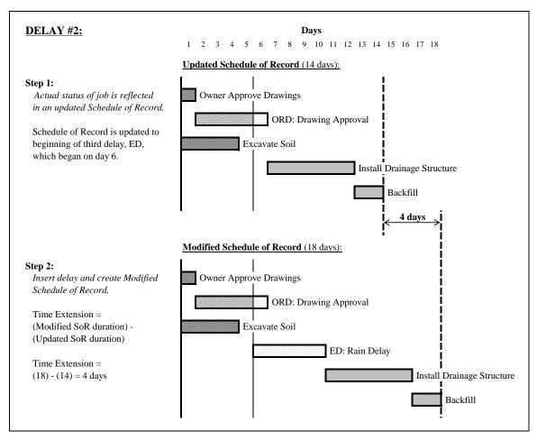
Figure 20: Modification Impact Analysis (U.S. Army Corps of Engineers') Approach
