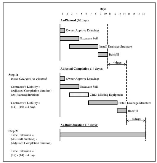
Figure 16: Adjusted As-Planned CPM Approach
