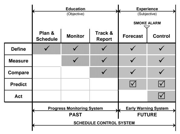
Figure 2: Structure of a Schedule Control System
