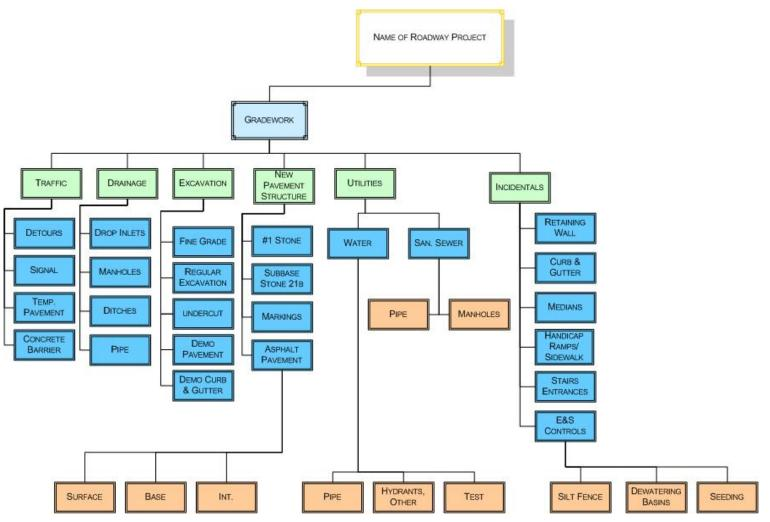
Figure 4: Typical WBS for Roadway Construction
