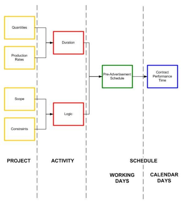
Figure 2. General Contract Time Determination Process flowchart
