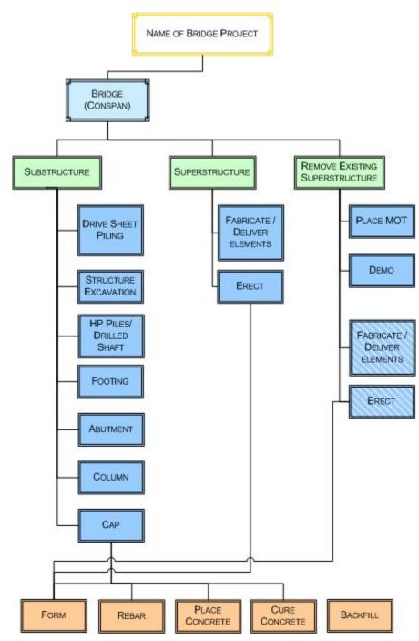
Figure 5: Typical WBS for Bridge Construction
