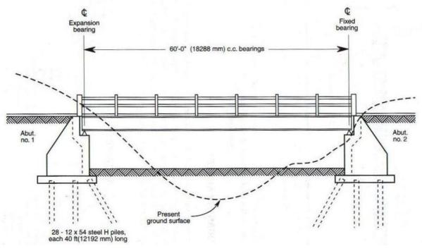
Figure 5: Highway Bridge Profile (Clough et al. 2000)
