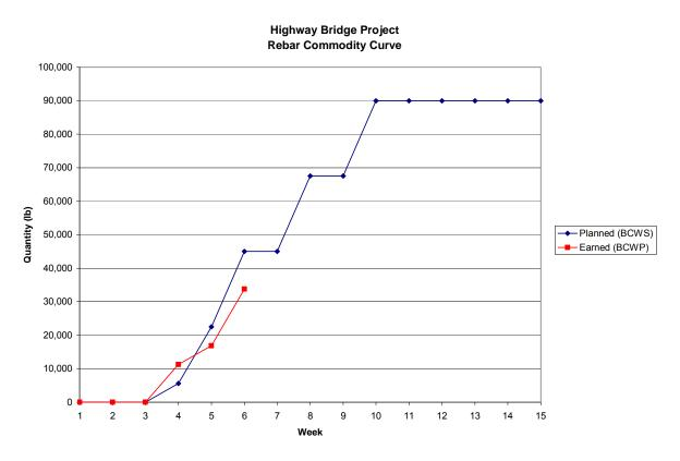
Figure 12: Commodity Curve for Rebar in Week 6
