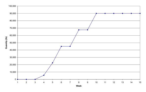
Figure 8: Commodity Curve for Planned Rebar Progress
