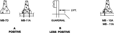
Barrier may require anchoring to the pavement or bolting to the bridge deck. Refer to Section 3, Barrier Design Considerations, for additional guidance. If anchoring/bolting is required it shall be on the traffic side(s) of the barrier. All barriers shall be installed in accordance with Section 500 of the current Road and Bridge Standards.
