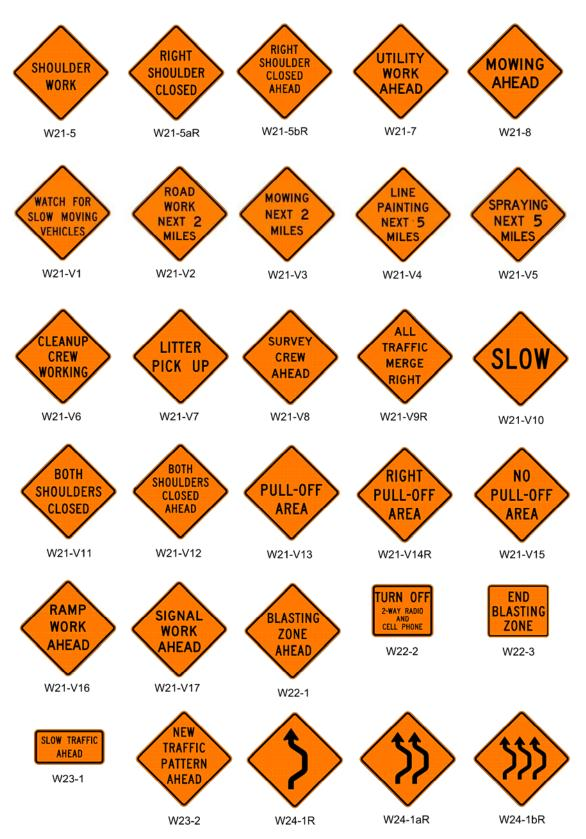
Figure 6F-3, Warning Signs and Plaques in Temporary Traffic Control (Sheet 5 of 5)<sup>1</sup>
