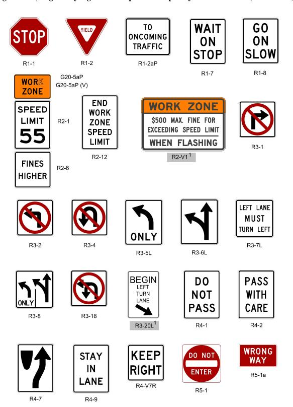
Figure 6F-2, Regulatory Signs and Plaques in Temporary Traffic Control (Sheet 2 of 2)
