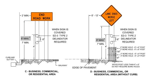
NOTE: FOR POST SIZE & INSTALLATION PROCEDURES SEE EITHER THE PLAN INSERTABLE SHEET OR VIRGINIA ROAD AND BRIDGE STANDARDS WSP-1 & ED-3 OR TEMPORARY SIGNS. <sup>1</sup>
