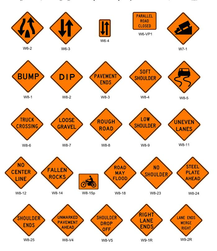
Figure 6F-3, Warning Signs and Plaques in Temporary Traffic Control (Sheet 3 of 5)<sup>1</sup>
