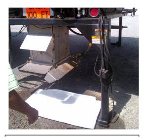
Oil absorbent pad attached to plywood
