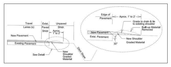
Figure 2: Wedge over Existing Pavement – High Shoulder
