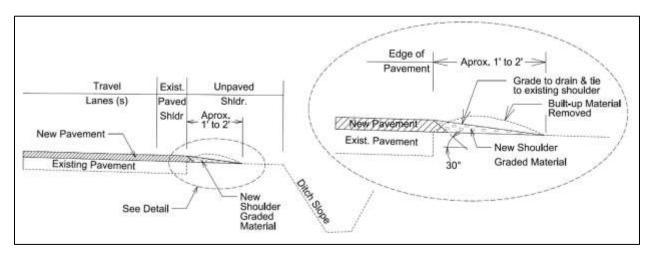
Figure 4: Wedge over Unpaved Shoulder – High Shoulder
