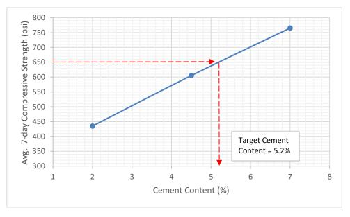
Figure 1: Example compressive strength versus cement content graph
