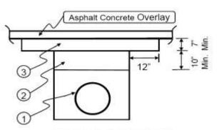
PAVEMENT STRUCTURE Scheduled for Asphalt Conc. Overlay
