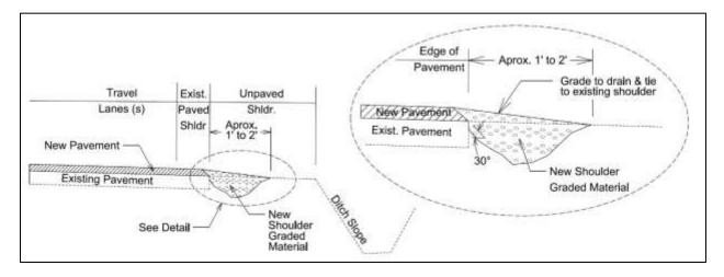
Figure 1: Wedge over Existing Pavement – Low Shoulder
