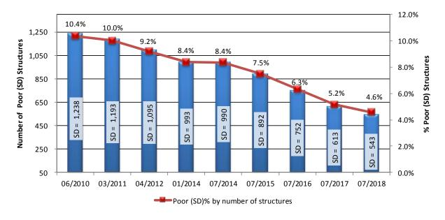
Figure 3-23- Percentage of Poor (SD) Structures - Recent Trends for Secondary System
