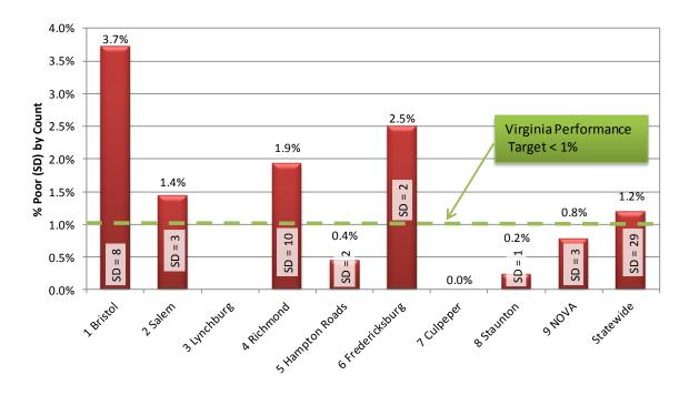
Figure 3-10- Percentage and Count of Poor (SD) Structures on Interstate System by District
