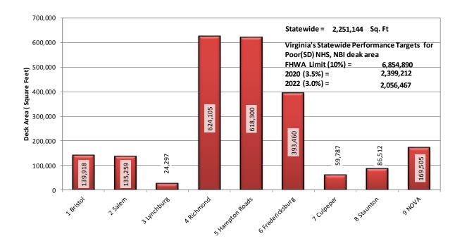
Figure 3-15- Deck Area of Poor (SD) NBI Structures on NHS by District
