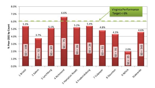
Figure 3-12- Percentage and Count of Poor (SD) Structures on Secondary System by District
