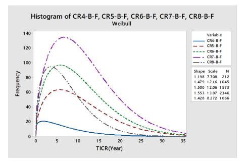
Figure 5- Probability Density Function Substructure GCRs for Bridges with Steel Girders and a Concrete Deck
