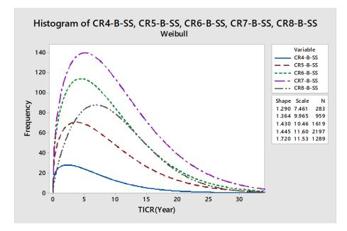
Figure 4- Probability Density Function for Superstructure GCRs for Bridges with Steel Girders and a Concrete Deck
