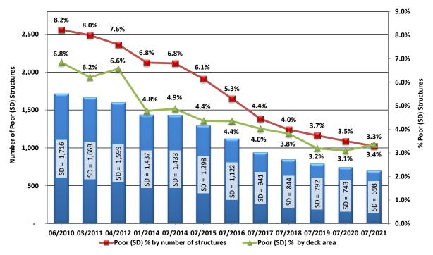
Figure 1: Multi-Year Performance History of Poor (Formerly Referred to as Structurally Deficient) Structures on All Systems
