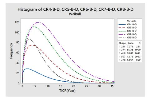
Figure 3- Probability Density Function for Deck GCRs for Bridges with Steel Girders and a Concrete Deck
