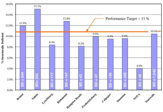
Chart 12 - Percentage of Structurally Deficient Structures – Secondary End of FY 2011
