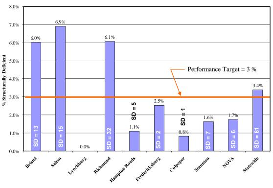
Chart 8 - Percentage of Structurally Deficient Structures – Interstate End of FY 2011
