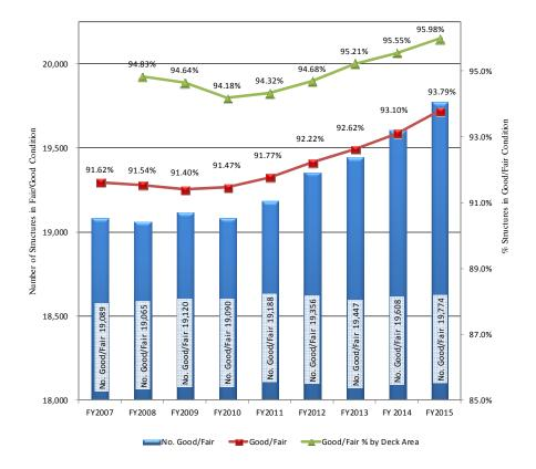
In addition to the percentage of SD structures, VDOT also tracks other indicators to assist in the overall management of the structural inventory. These include: functional obsolescence (FO), structurally deficient structures, the number of posted structures, deficient deck area and the Health Index.
