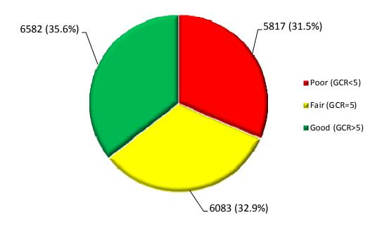
Chart 15e provides the condition of the ancillary structures by structural component by asset statewide. In Appendix K, other charts are presented to gain a more specific understanding of the conditions that cause structures to receive reduced GCRs.
