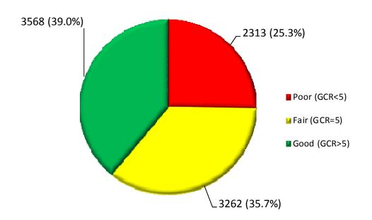
Chart 15c - High Mast Lights and Camera Poles by Minimum General Condition Rating
