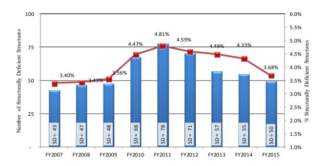
Chart D.11 – Percentage of Number of NHS (Only NBI) Structurally Deficient Structures on Interstate System at End of FY 2015
