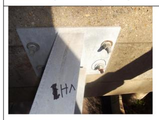
Failed mounting bolt (circled)
