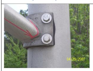
Lower arm of luminaire chord has a 3.5" fatigue crack in weld at connection to pole
