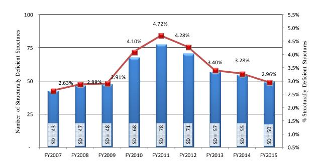
Chart D.12 – Percentage of Number of NHS (Only NBI) Structurally Deficient Structures on Primary System at End of FY 2015
