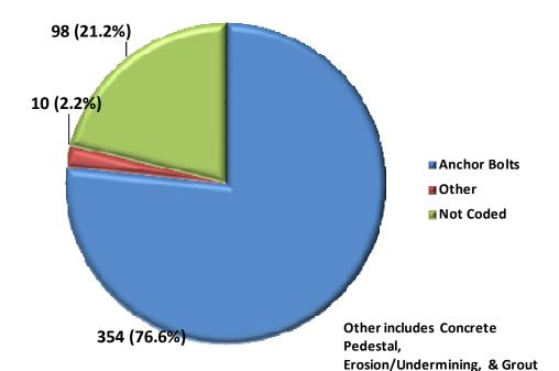
Chart K.2.a – Reasons Coded for Poor Sign Structure Foundation
