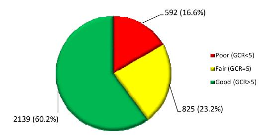
Chart 15b – Signal Structures by Minimum General Condition Rating
