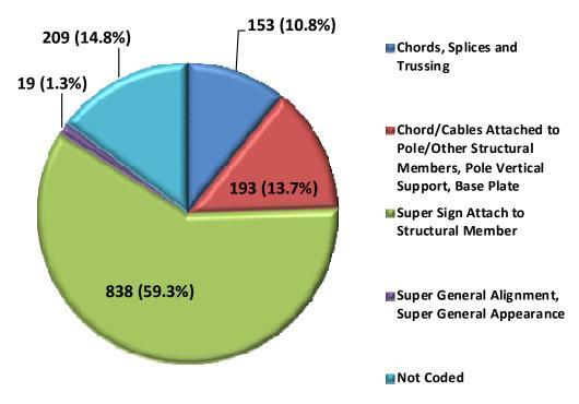
Chart K.5.a – Reasons Coded for Poor High Mast Light and Camera Poles Foundation
