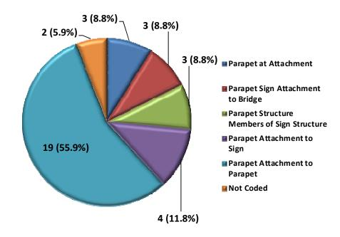
Chart K.2.c – Reasons Coded for Poor Sign Structure Superstructure
