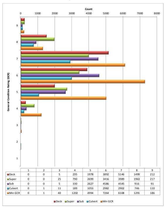
The Min GCR represents the minimum or lowest General Condition Rating (GCR) for the structure (lowest of the 4 component ratings for a particular inspection report; deck, superstructure, substructure, or large culvert)
