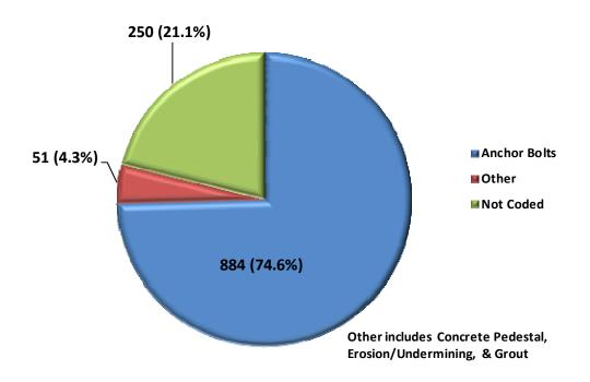
Chart K.4.b – Reasons Coded for Poor Signal Structure Superstructure
