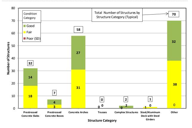
Figure 2-9- Count and Condition Data for Less Common Structure Categories (Non-NBI Structures)
