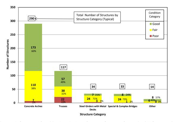
Figure 2-5- Count and Condition Data for Less Common Structure Categories (All Structures)
