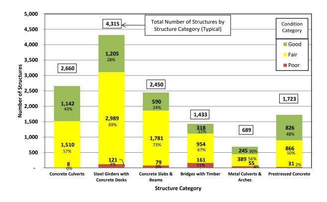
Figure 2-6- Count and Condition Data for Most Common Structure Categories (NBI Structures)
