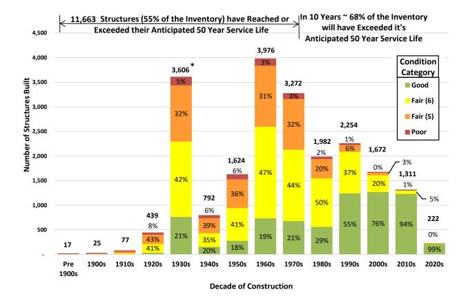
Figure 2-3- Count of Structures Built by Decade and Condition Percentage by Count
