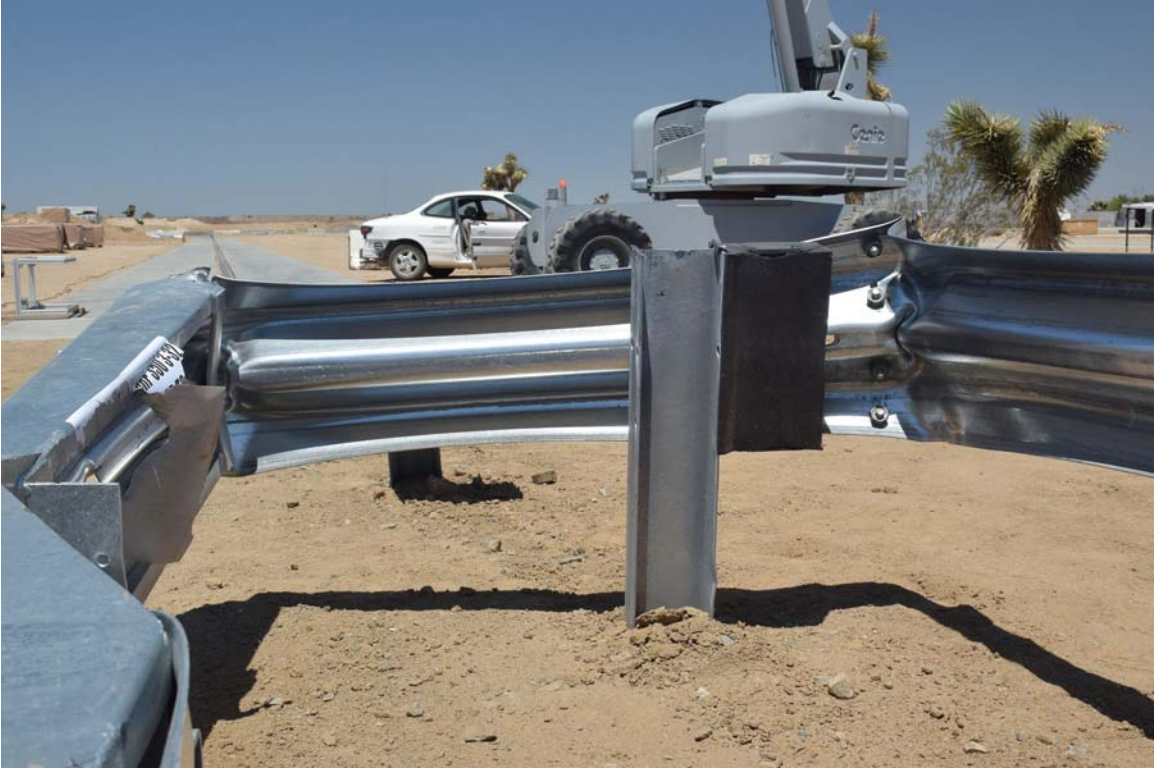
FIGURE 37. Test Article Damage
