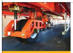
New Program Speeds Pavement Testing VDOT and the Virginia Tech Transportation Institute unveiled their new joint "accelerated pavement testing" program in November. A "heavy vehicle simulator," the technological heart of the program, will cut years off the time needed to test how new pavement designs and mixes perform under the daily impacts of heavy traffic.
