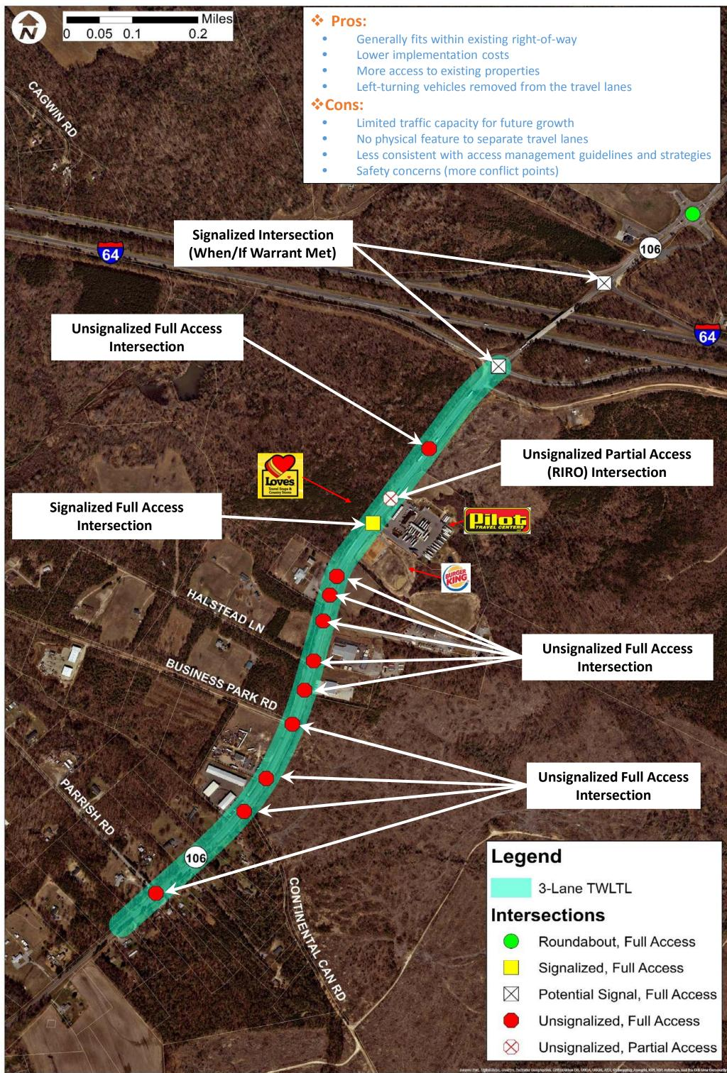
Figure Route 106 Arterial Management Plan **Three-Lane Typical Access** Kimley »Horn Management Scenario New Kent County, VA 24
