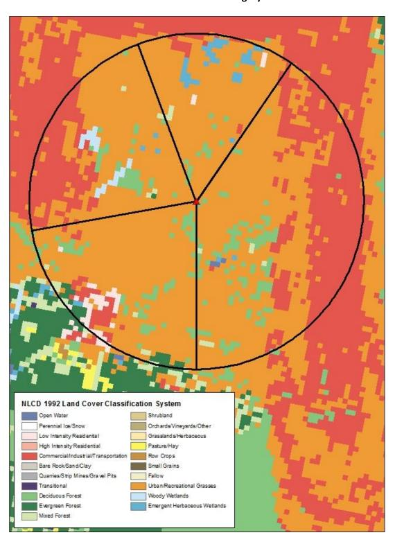
Figure 2: 1-Km Radius for Dulles International Airport with Surface Roughness Sectors
