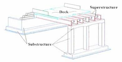
Structural elements of a typical highway bridge
