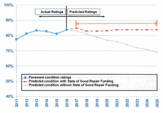
Figure 33: Previous and Forecasted Pavement Condition (Percent Sufficient) - Primary
