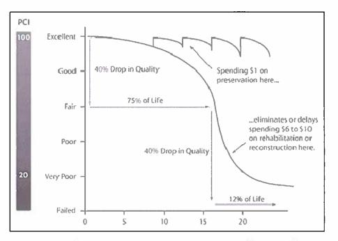
Figure 2: Impact of Maintenance Timing on Asset Condition
