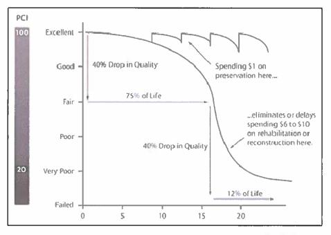
Figure 40: Impact of Maintenance Timing on Asset Condition
